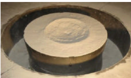
A 30cm-diameter crater plus spattered dust are all that's left after a test shot in the Ames Vertical Gun. Photo credit: NASA.
