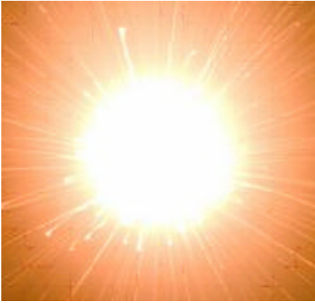
Death of a shooter. This is a real photo of a pyrex marble exploding on impact at the NASA Ames Vertical Gun Range. Photo credit: Peter Schultz, Brown University, and NASA
